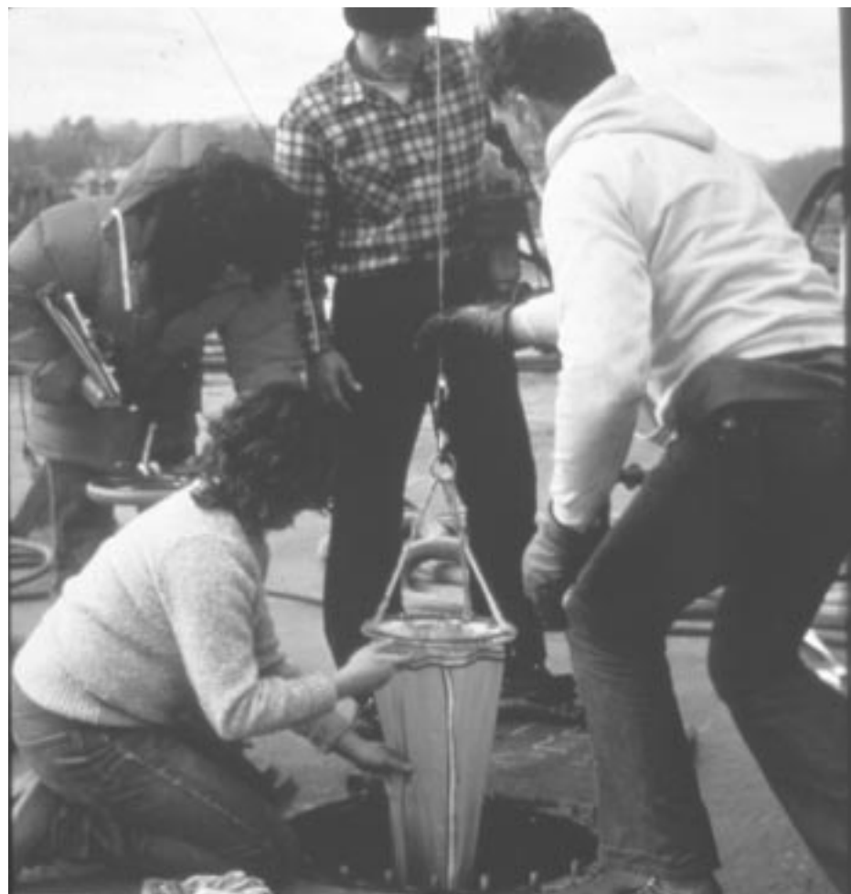
Plankton sampling can reveal the kinds of organisms ballast water contains. Researchers are exploring ways to treat ballast water before it is discharged — including filtration, heat, and irradiation — to kill exotic organisms that could invade coastal areas.
