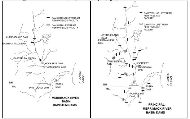
Figure 11-2 Mainstem (left) and Principle (right) Merrimack River Basin Dams
