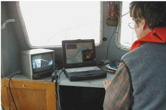
Survey Operations Showing use of RoxAnn™ and real-time video of sea floor (image courtesy of Maine Department of Marine Resources).
