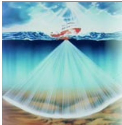
Figure 1. Vessel with multibeam sonar array maps a swath of seabed (courtesy of Simrad).
