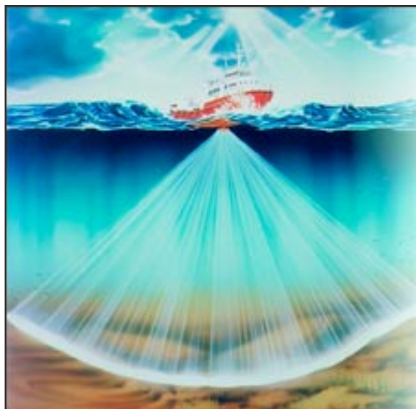
FIGURE 4. Diagram showing the swath coverage of multibeam sonar soundings used to map the sea floor. Courtesy of Simrad.
